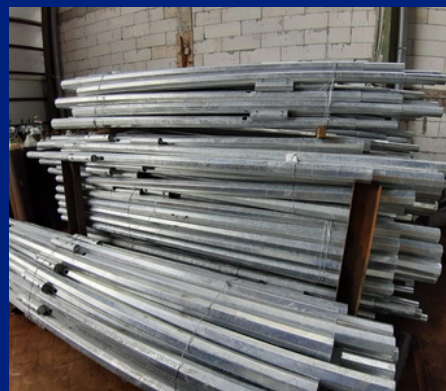
Tiang PJU Solar Panel
